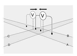
The principle of operation of the 'A' frame is the same as described above except that it does not use a DC battery. In practice, the battery idea does not work because of stray naturally occurring ground currents overpowering the weak fault current. Instead, ac signals are used. The receiver's circuitry decodes the information contained in the signal in order to display the relative direction of flow.
