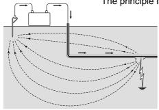
Sheath or coating faults are detected with an 'A' frame accessory for the receiver.
