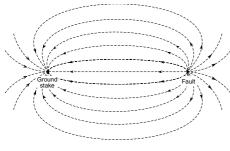
At the sheath fault, the current is 'escaping' to ground and will immediately spread out and return to the battery via many different routes.
