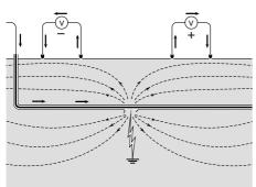
If a voltmeter is connected to the ground at two points, as illustrated, it will display a positive reading or a negative reading, depending on the direction of flow of the local ground currents.
