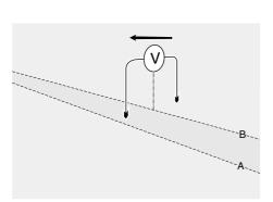
Note that the meter does not indicate directly the direction of the fault. Imagine a line drawn through the centre of the meter; the meter deflection indicates which side of the line the fault is.
