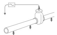
Direct connection: The output ac voltage from the signal transmitter is connected directly to the pipe or cable at an access point such as a valve, meter or end of the conductor, and the circuit is completed by a connection to a stake or other ground connection point.
