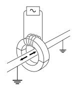
Clamping the signal: Clamping uses the induction principle to give a similar result to direct connection, but without electrical contact to the line. The output from the signal transmitter is applied to a target line by clamping round it with a split toroidal magnetic core, which carries a primary winding magnetizing the core with the ac signal. The line becomes the secondary of a transformer, and will carry a strong signal, provided that it is adequately grounded on each side.
