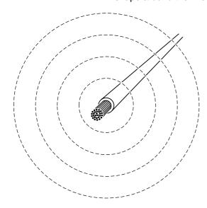
While it is possible to insulate against the flow of electricity it is not possible to insulate against a magnetic field, and the shape of the field is not changed by cable insulation or by the presence of different types of soil.
