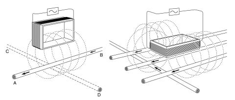
In the first drawing the transmitter aerial lies parallel to line AB and its field links around the line which therefore has a signal induced on it. There is no linkage and no signal induced on line CD at right angles to the aerial.
