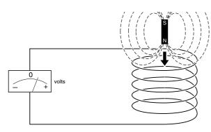
The principal of electromagnetic induction can be illustrated by inserting a bar magnet into a coil of wire. The voltmeter will show a deflection but only while the magnet is moving.
